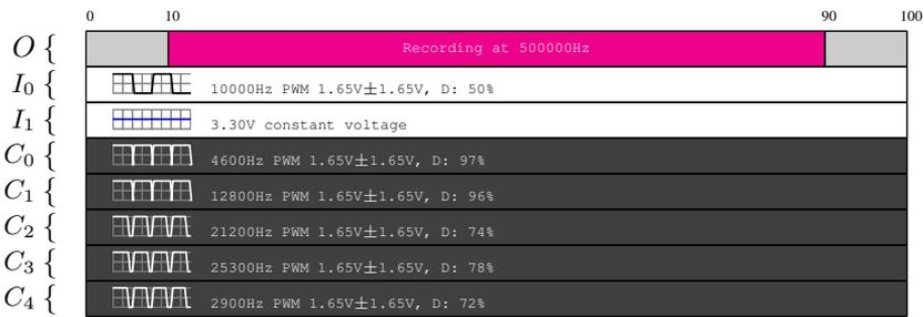
**Figure 3.12:** Timing overview of the activity on each logical electrode over time during a single computation of  $1 \vee 0$  on the evolved OR gate. Time progresses along the x-axis, labeled in milliseconds at points of interest.  $O$  is the output pin,  $I_n$  are the input pins, and  $C_n$  are the configuration pins. The small waveform illustrations reflect the duty cycle, but not the frequency.  $D$  is the duty cycle.
