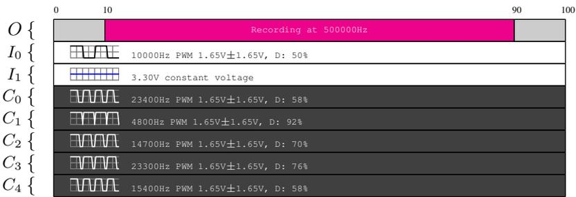
**Figure 3.10:** Timing overview of the activity on each logical electrode over time during a single computation of  $1 \wedge 0$  on the evolved AND gate. Time progresses along the x-axis, labeled in milliseconds at points of interest.  $O$  is the output pin,  $I_n$  are the input pins, and  $C_n$  are the configuration pins. The small waveform illustrations reflect the duty cycle, but not the frequency.  $D$  is the duty cycle.
