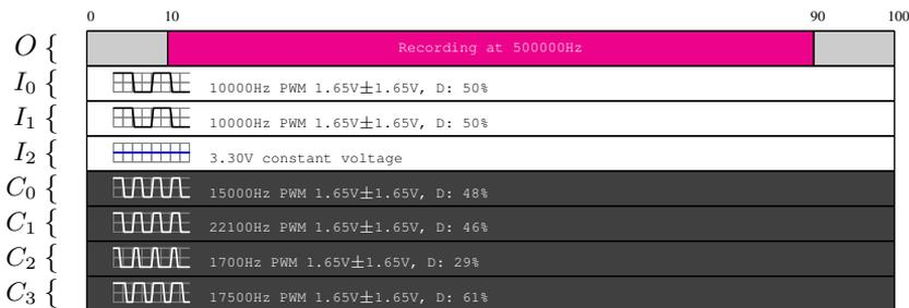
**Figure 3.17:** A timing overview of the activity on each logical electrode over time during a single computation of  $r151(011_2)$  on the evolved Rule 151 device. Consult the Figure 3.16 caption for a legend.
