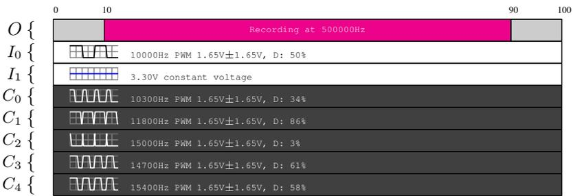
**Figure 3.14:** Timing overview of the activity on each logical electrode over time during a single computation of  $1 \oplus 0$  on the evolved XOR gate. Time progresses along the x-axis, labeled in milliseconds at points of interest.  $O$  is the output pin,  $I_n$  are the input pins, and  $C_n$  are the configuration pins. The small waveform illustrations reflect the duty cycle, but not the frequency.  $D$  is the duty cycle.
